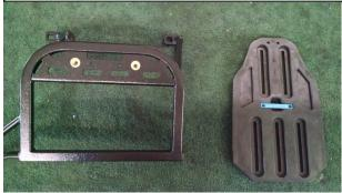
Step 1, Attach the Mosko plate to the Non-tool plate side of the SU rack OR SL rack (see notes):
