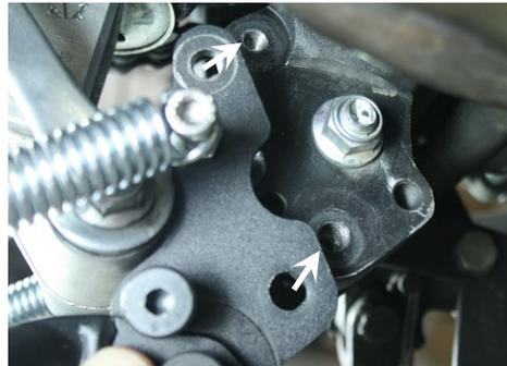
Place a 8mm star washer and flat washer onto the 8mm bolt. Using one hand, lift the center stand into position, aligning the mounting holes on the center stand with the mounting holes on the frame. Unlike the previous side, insert the 10mm bolt into the BOTTOM mounting hole on the center stand first. Slide on one 16mm long (5/8") spacer and any necessary extra flat washers to fill the gap behind the bolt and thread it into the hole by hand.
