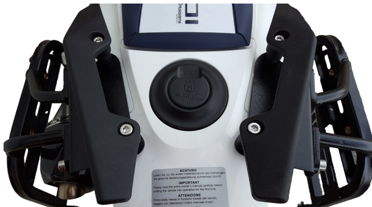
Figure 5: Top view of installed grab handles and rack 2
