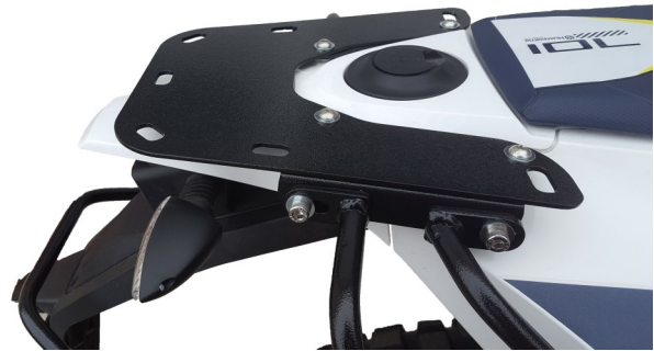
Figure 4: The top plate mounted with the SU rack.
