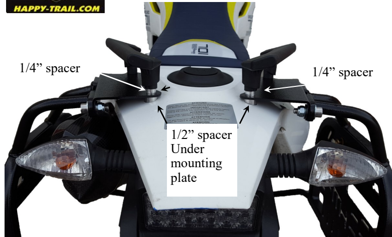
Figure 3: Rear picture showing the grab handles mounted on top of the SU mounting plates.
