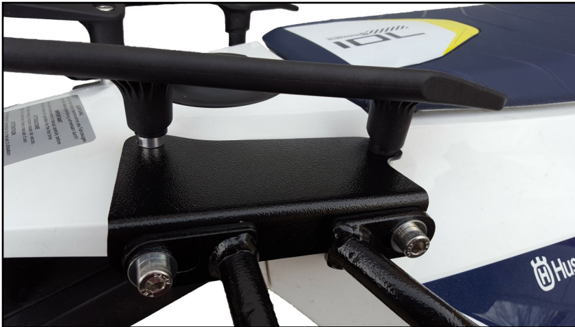
Figure 6: The SU top rear and top front mounts attached to the mounting plates.
