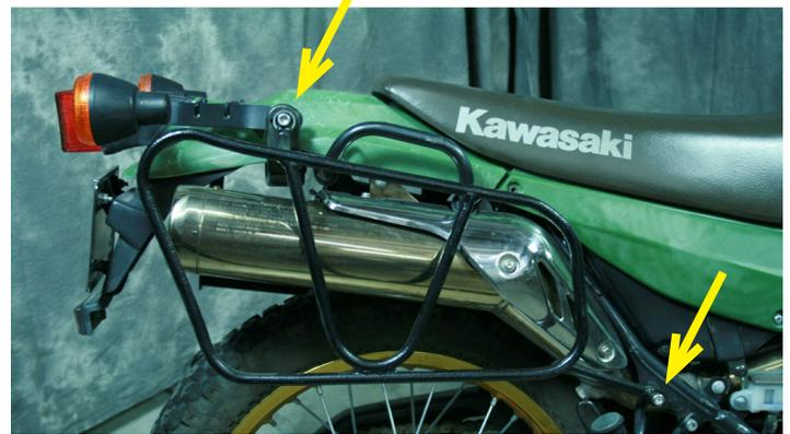
**NOTE 1:** The turn signal wiring has a factory supplied disconnect point hidden between the exterior (green color) and interior (black color) rear fenders. To take advantage of the supplied wiring disconnect you need to remove the exterior fender to access the wiring disconnect point.
