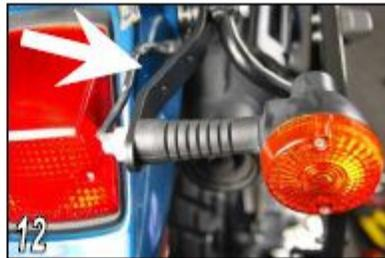
Using the black nylon spacer at the rear rack mounting location (pic 11), and the white spacer at the end with the turn signal (pic 10) attach the turn signal to the end of the tab with the one big hole and two small holes.
