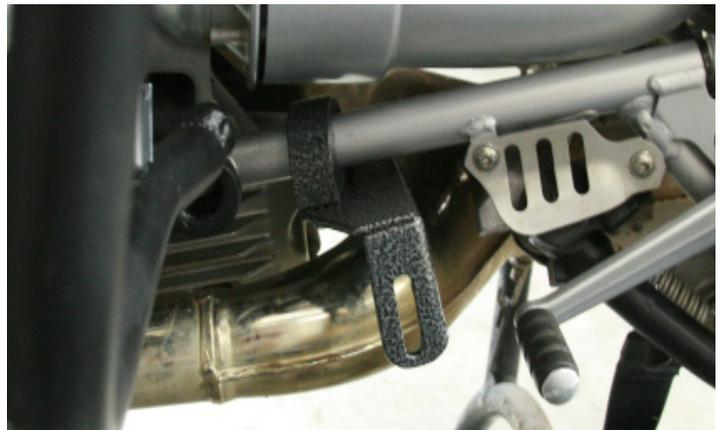
Place an M6 Lock Washer onto the M616C bolts, place an M6 flat washer on the bolts, then slide the bolts through the slot in the L bracket and thread into the U clamp installed in Step 4. Do not tighten yet.
