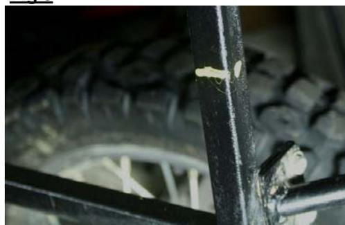
Users with larger drills will need to mark an additional hole on the outside of the SU Rack frame. Draw a line out the outside of the SU Rack as shown in Fig 3. Place an additional felt pen or paint pen mark on the outside of the SU rack on all three mounting holes.
