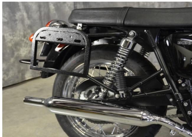
Replace seat and two bolts at back to complete install.
