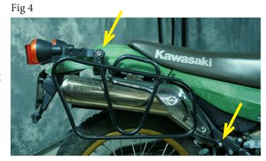
**NOTE 1:** The turn signal wiring has a factory supplied disconnect point hidden between the exterior (green color) and interior (black color) rear fenders. To take advantage of the supplied wiring disconnect you need to remove the exterior fender to access the wiring disconnect point.
